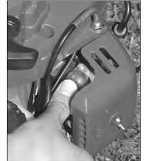
**NOTE: Don't press the throttle trigger during the starting of the engine.**
