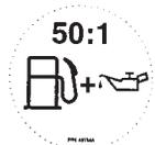
Mix unleaded gas with 2 cycle 50:1 oil. Must meet or exceed ISO-L-EGD (ISO/CD13738) and J.A.S.O. FD Standards
