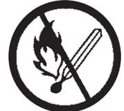
DON'T FUEL, REFUEL, OR CHECK FUEL WHILE SMOKING, OR NEAR AN OPEN FLAME OR OTHER IGNITION SOURCE.
