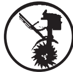
CAUTION: WHEN ASSEMBLING THE HANDLES, MAKE SURE FUEL TANK FACES OPERATOR. THIS IS THE REAR OF THE TILLER, REFER TO ASSEMBLY INSTRUCTION ON PAGE 7.
