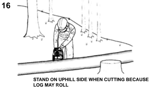
When bucking on a slope always stand on the uphill side of the log, as illustrated in Figure 16. When "cutting through", to maintain complete control release the cutting pressure near the end of the cut without relaxing your grip on the chainsaw handles. Don't let the chain contact the ground. After completing the cut, wait for the saw chain to stop before you move the chainsaw. Always stop the motor before moving from tree to tree.
