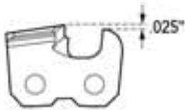
The depth-gauge setting for all square-ground chisel chain is  $.025$ ".
