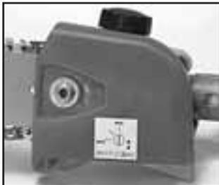
3. Move saw chain backwards on guide bar by hand. Saw chain should move freely on guide bar if it is in proper mesh with the sprocket. If saw chain is difficult to rotate or binds on guide bar, it is too tight. Re-adjust if necessary.
