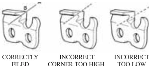
To properly sharpen the cutter, use the correct filing position, as shown here from three different points of view:
