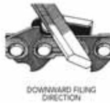
The chain manufacturer recommends that square-ground chain be filed from the outside in (in a downward direction). This leaves a better edge on the chromed cutting surfaces and makes it easier to keep the file's position, and the resulting cutting edges, in correct alignment as
