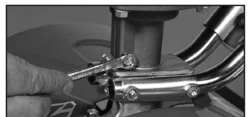
Picture 4. Note how the engine sits all the way down on the transmission.
